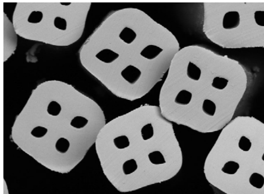
Antron® type 6,6 nylon hollow filament
