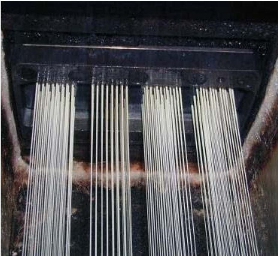
Fiber Shape determined by Spinneret
